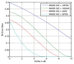
Figure 3: BER performance comparison of downlink DAS Group Cell processing scheme aided MIMO OFDMA wireless communication system with adaptation of MMSE-SIC signal detection and various Digital modulation schemes
