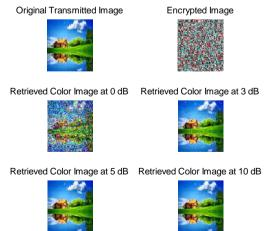
Fig. 7 Transmitted, Encrypted and Retrieved color images at various SNR values in a downlink DAS Group Cell
