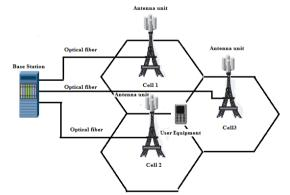
Fig. 1 Scenario of Distributed Antenna Systems (DAS) with multiple remote antennas connected to a single Base Station (BS)
