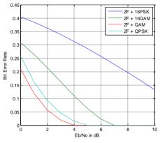
Fig. 4 BER performance comparison of downlink DAS Group Cell processing scheme aided MIMO OFDMA wireless communication system with adaptation of ZF signal detection and various Digital modulation schemes
