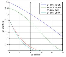
Fig. 5 BER performance comparison of downlink DAS Group Cell processing scheme aided MIMO OFDMA wireless communication system with adaptation of ZF-SIC signal detection and various Digital modulation schemes
