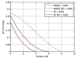
Fig. 6 BER performance comparison of downlink DAS Group Cell processing scheme aided MIMO OFDMA wireless communication system with adaptation of QAM digital modulation and various signal detection schemes
