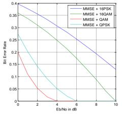
Fig. 2 BER performance comparison of downlink DAS Group Cell processing scheme aided MIMO OFDMA Wireless Communication System with adaptation of MMSE signal detection and various Digital modulation schemes
